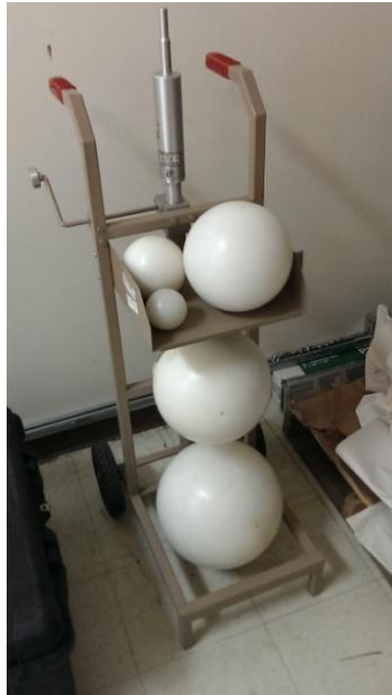
Figure 19. Sample setup of the BSS using the transport cart as a measurement apparatus with the bare scintillator atop the cart.
